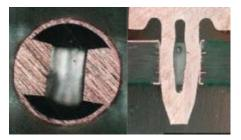
Direct Connect to PCB hole (no solder voids)
