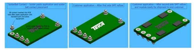
For end manufacturers, because solder ball-enabled modules automatically adjust for co-planarity variances during reflow, the manufacturer gains significant latitude in the process window. Instead of needing to be sure that all of the module contacts are perfectly seated during placement, they can rely on the automatic compensation of the solder balls to close gaps and provide 100% solderability.
