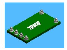
In the electronics industry, the term "co-planarity" typically refers to the maximum distance that the physical contact points of a surface-mount device (SMD) can be from its seating plane. When placed on a flat surface, an SMD device or module will rest on its three lowest points. This is the seating plane of the device. The co-planarity specification defines the maximum gap that can exist from the underside of any pin to the PCB to which it is being soldered.
