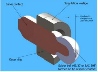
Normally device co-planarity has a specification of .01mm max. The device sits on the highest leads (3 minimum) and then all other leads can be no more than 0.1mm off the PCB surface. The solder ball contact allows that co-planarity limit to increase a by a minimum of 4 times to over 0.4mm.
