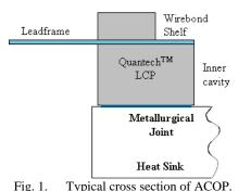
The first step in the package assembly process is to bond the window frame to the heat sink (Fig. 2). The Quantech<sup>TM</sup> material is formulated to withstand the high temperature rigors of the hard solder attachment while the bond between the Quantech<sup>TM</sup> window frame and metallic interfaces are not compromised.
