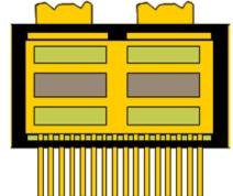
Fig. 2. Schematic of die bonded ACOP-18L prior to lid attach
