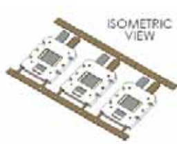
Figure 4. A CPV package unit on leadframe carrier.
